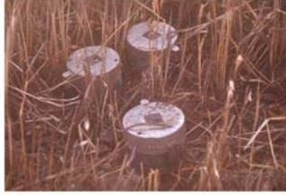
Picture 7: Three submunitions closely grouped. The specialist I interviewed commented: *“The BLU108 warheads were generally grouped together in groups of four and a few sites showed evidence of warhead detonations amongst unexploded warheads. These detonations appear to have occurred on impact rather than target acquisition and fuse detonation above the target”*
